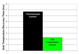
**Figure 2** displays an average of the time required for gob temperatures to stabilize after a job change.
