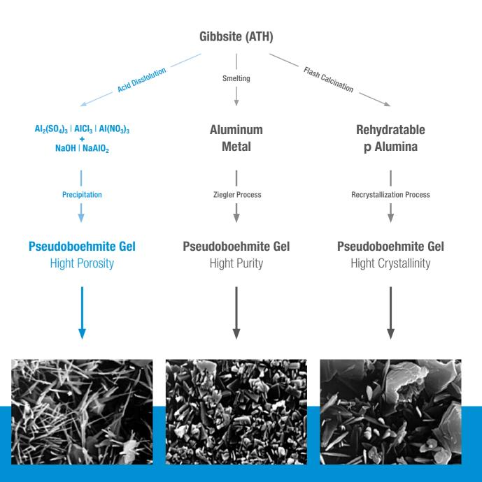
Different aluminas are chosen based on their different properties and applications. Properties such as porosity, purity, surface area, and density should be considered when choosing an alumina.
